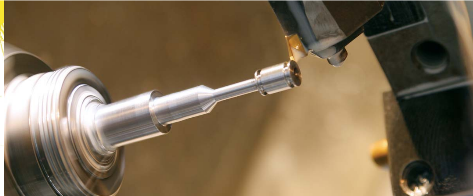
DYE guns require a number of precision turned parts. Here, a DM5 fuse-bolt nears completion. The use of bar feeders on their Haas lathes keeps production flowing.
